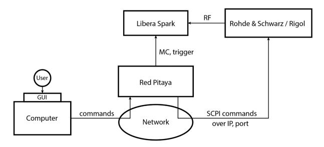
The user has to connect to Red Pitaya's web application over a computer that is in the same network. The GUI is accessible in a browser: rp-<last 6 digits of MAC address>.local
